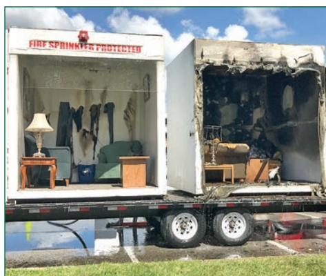
EH&S hosted a fire demonstration showing the benefit of having fire sprinkler protection. The room on the right had no sprinkler protection and was engulfed in flames in under one minute. The room on the left was sprinkler protected and the fire was extinguished within seven seconds, with minimal damage.
