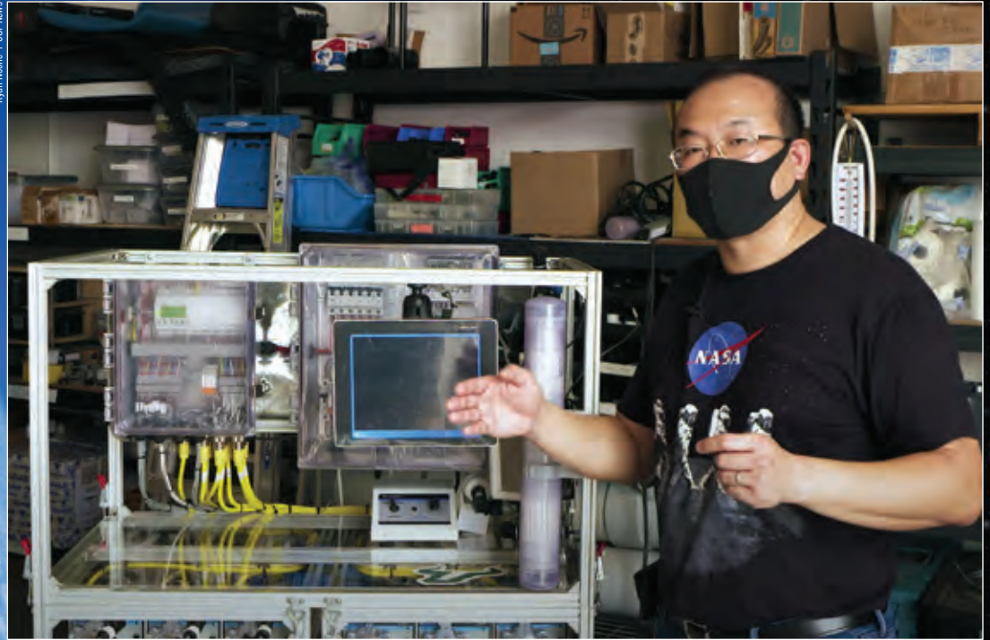
Above: Civil and Environmental Engineering Professor Daniel Yeh demonstrates the Organic Processor Assembly, a system that extracts nutrients from human waste.
