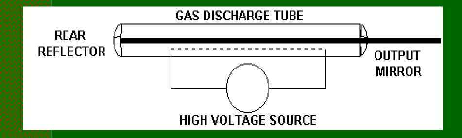
Gas lasers consist of a gas filled tube placed in the laser cavity. A voltage (the external pump source) is applied to the tube to excite the atoms in the gas to a population inversion. The light emitted from this type of laser is normally continuous wave (CW).
