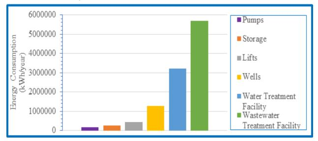
Figure 6. 2017 Energy Consumption of Water Transfer Components
