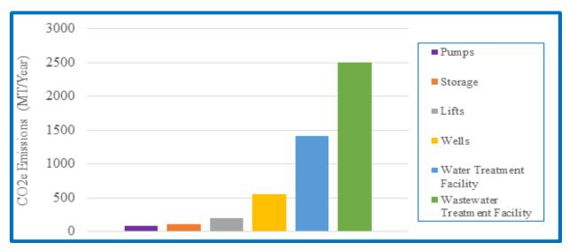
Figure 7. 2017 CO<sub>2</sub> Equivalent Emissions from Water Transfer Components
