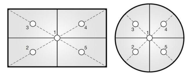
The test load used in an eccentricity test **should be within the range** of the weighing instrument and preferably using just one test load. That way it is easier to be sure that the load's center of gravity is in the specified location. For a weighing instrument with multiple ranges, the eccentricity test should be done with the highest range.
