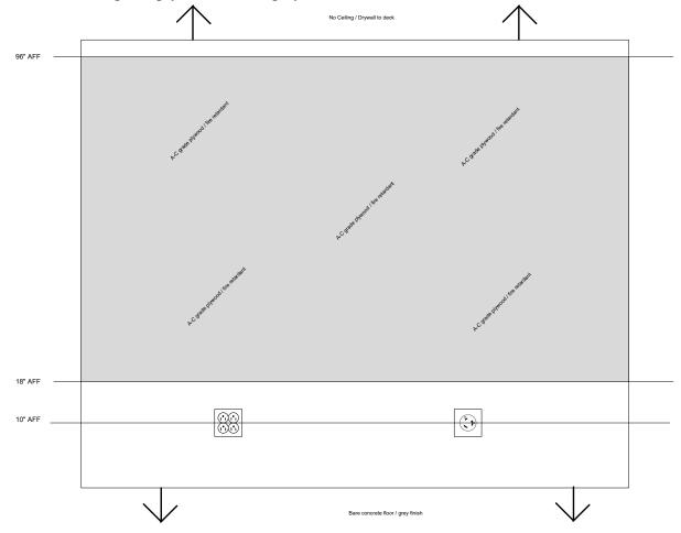
TR and EF floors shall be finished with sealed or painted concrete floors, color gray.
