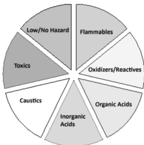
Figure 1: Sample Chemical Storage Scheme
