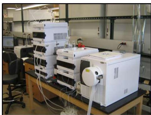
Figure: Agilent 6120 LC/MS (left) and chromatogram (right) of compounds isolated (highlighted in blue) by mass-based collection.
