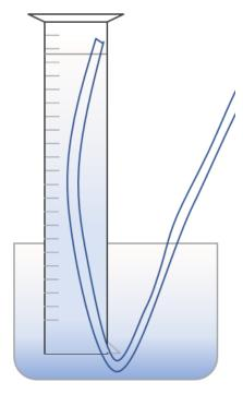
If rubber bands are unavailable, you may choose to drill holes in the base of the graduated cylinder and the water bath (if they are plastic). If the biogas is being collected in heavy glassware, it probably isn't necessary to stabilize the system. However, the tubing needs to be inserted before flipping the glassware down into the water bath.
