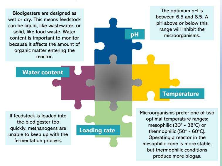
Some control factors are easily measured, such as the loading rate and the temperature of the reactor. Other factors must be measured to ensure the operators are aware of issues *before* reactor souring occurs:
