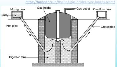
The steel drum can be expensive, but it is easier to install than a fixed dome. The drums are smaller than a dome, so they cannot hold as much biogas. Like the fixed dome reactor, feedstock enters through the inlet and digestate comes from the outlet pipes.
