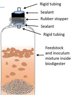
This part of the experiment is flexible and can be changed with the adaptations given earlier in the chapter. For instance, the bottle's original lid may be used instead of a rubber stopper, but it could be more challenging to puncture.
