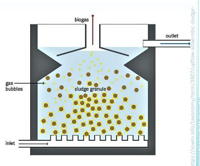
This technology can be applied to many types of reactors with different mechanisms. Pictured here is an Upflow Anaerobic Sludge Blanket Reactor, where effluent is piped to the bottom of a large tank. As it flows upwards, it is filtered by a blanket of anaerobic microorganisms, which convert the organic matter to biogas. The treated sludge can be safely disposed of.
