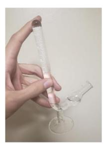
It may be a good idea to practice this procedure with water before using biogas and a strong base. It can be tricky to fill up the fermentation tube completely, and also to inject the gas all the way into the tube without it leaking out. Simply inject air into the fermentation tube, filled with water, trying to keep all the bubbles within the tube.
