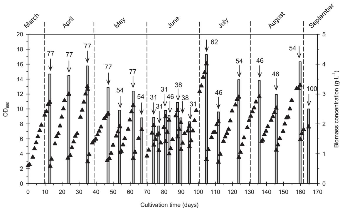
**Fig. 5.** Cultivation of *N. atomus* in the floating 65-L HBR during outdoor semi-continuous operation in central Florida. Daily growth as monitored by  $\text{OD}_{680}$  ( $\blacktriangle$ ); arrows and their adjacent labels mark culture harvesting and % of total reactor volume harvested, respectively; gray bars show the biomass concentration at harvest.
