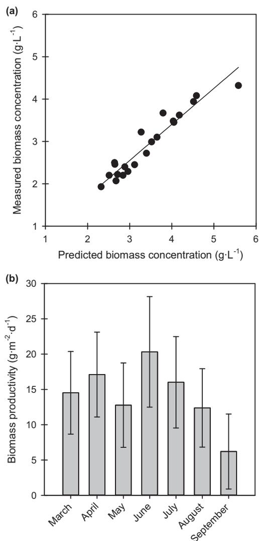
**Fig. 6.** (a) Linear correlation between biomass concentration predicted from OD–DCW indoor correlations and measured biomass concentration outdoors at harvest; (b) Monthly biomass areal productivity ( $\text{g m}^{-2} \text{d}^{-1}$ ) in the floating 65-L HBR during outdoor semi-continuous cultivation of *N. atomus* in central Florida. Average productivities are shown ( $n=2-26$ ) with the error bars denoting standard deviation.
