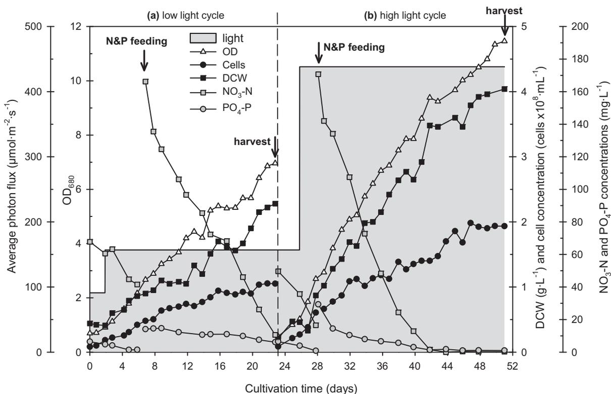
**Fig. 3.** Growth and nutrient consumption of *N. atomus* during the two cultivation cycles, 0–23rd day and 23rd–52nd day, in the floating HBR under two artificial illumination levels of (a) 11.3 klux and (b) 31.1 klux. After the 1st cycle (growth in low light) 90% (v/v) of the culture was harvested and the residual 10% (v/v) was used as inoculum for the 2nd cycle (growth in high light). The arrows mark either nutrient (nitrate and phosphate) feeding or culture harvesting.
