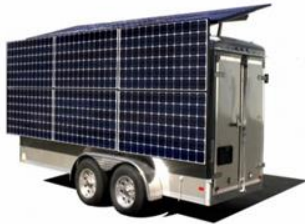
Figure 3. A solar power trailer that can house the mini plant [ http://www.mobilesolarpower.net/ ]
